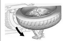
Lower the jack by turning the lug wrench counterclockwise. Keep lowering the jack until the spare tire slides off the jack.
